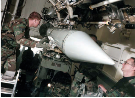
The B-61-11, often called an “aircarried” platform, is shown being loaded into a B-52 bomber.
