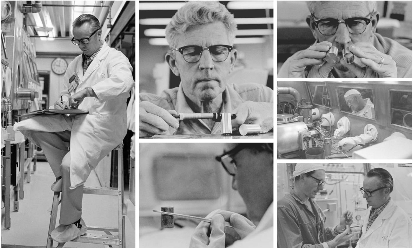
Clockwise from left: Larry Mullins records data during a direct oxide reduction experiment; Art Beaumont measures the outside diameter of a gauge tube with a micrometer; Beaumont compares a mock-up welded capsule and the gauge tube; Carl Peterson transfers plutonium oxide inside an inert-atmosphere glove box from a storage container in preparation for pressing a fuel pellet; Jim Foxx (left) and Larry Mullins discuss a helium release experiment with a vented plutonium-238 oxide heat source; the heat source capsule had to be handled inside a glove box with forceps because of the high temperature of the unit (generated by the alpha radioactive decay of plutonium-238).
